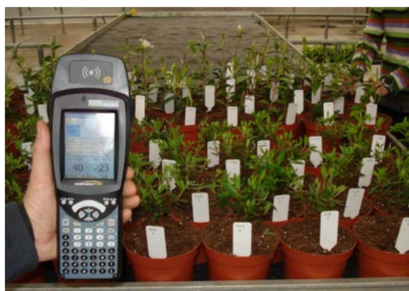
Figure 6. Psion Workabout Pro PDA reading 40 potted Camellia and Azalea electronically identified by means of plastic label UHF transponder.
