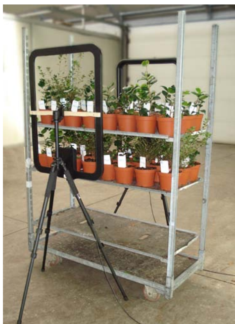
Figure 2. Multiple dynamic reading of 48 potted plants electronically identified by HF plastic label transponders.
